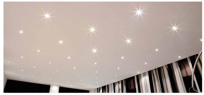
Flush-fitted in polished aluminium for accent, decoration and courtesy lighting. Also indicated for 'starry sky'. Choice of secondary optics, can be installed indoors and outdoors if partially protected, spring-mounted.
